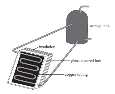
A solar water heater placed on the roof of a house consists of copper tubing placed inside a box and covered by a sheet of glass. The copper tubing is connected to a hot water storage tank. The cold water enters at the bottom of the solar heater and the hot water leaves from top of the heater.
